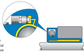
When the pressure screw is tightened to the recommended tightening torque, Tt, the steel ball seals against the spherical seating. ETP-TECHNO will create a uniform surface pressure against the shaft and hub.
